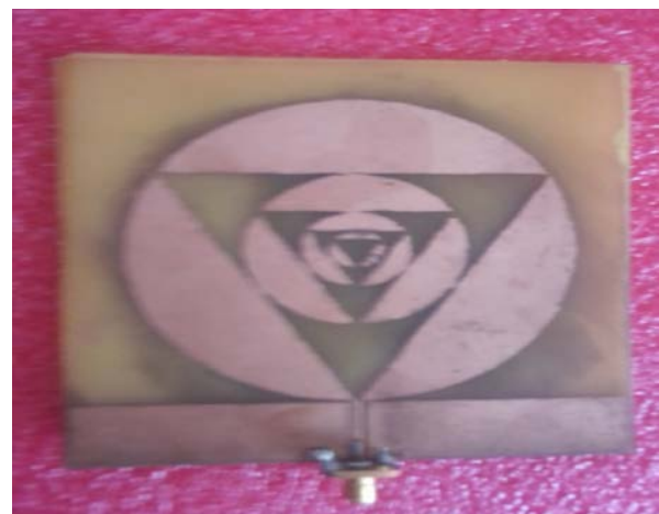
Fig 1. a) Fabricated UWB crown fractal antenna
