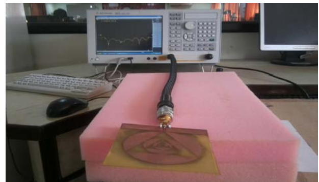
Fig.3 experimental setup for measuring parameters of a microstrip patch antenna
